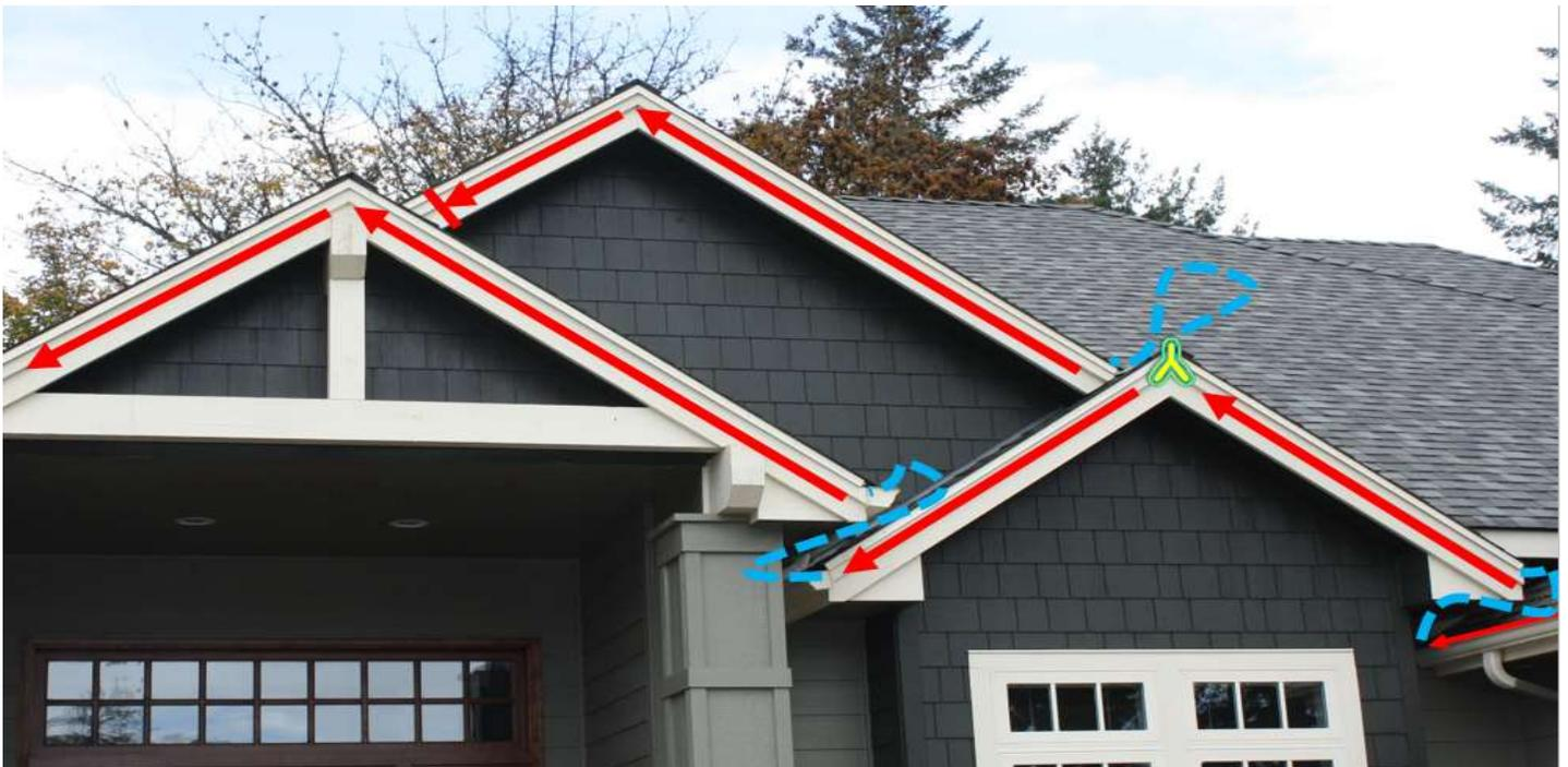
To help keep the chasing patterns moving sequentially in the right direction, there are some situations when it is best to add a Y-split at the peak of an eave. See diagram.
